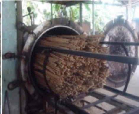
6: Bamboo bundles are steamed then dried in drying chamber
