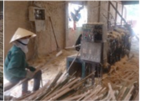
4: The bars of bamboo are scraped off and peeled
